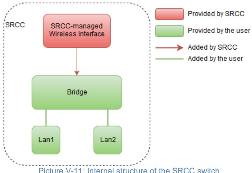
Picture V-11: Internal structure of the SRCC switch
