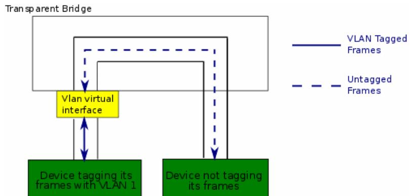
Picture V-7: VLAN tag conversion using a virtual interface
