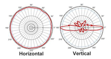
Typical Omni directional antenna radiation pattern (HG2415U-PRO)
