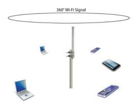
In the example above an Omni directional antenna is providing wireless connectivity for laptops, tablets, and smart phones in the coverage area.
