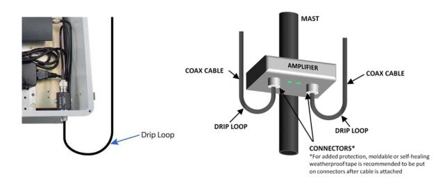
If you are using a wireless amplifier or radio it is best to position it as close to the antenna as possible (without putting too much stress on the connecting cables). Make sure the amplifier connectors are face down and leave enough room for drip loops.
