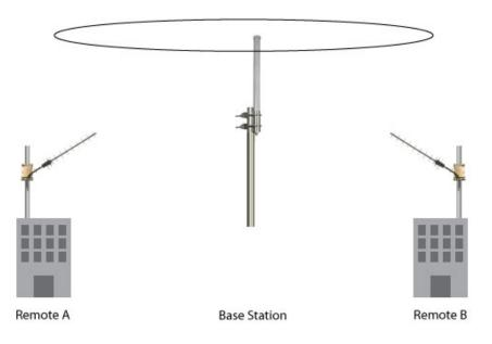
In this example both remote sites A and B have directional Wi-Fi connectivity to the base station fitted with an Omni directional antenna. This is an example of a point to multi-point set up.
