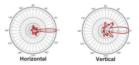
Typical Directional Antenna Radiation Pattern (HG2424EG-NF)
