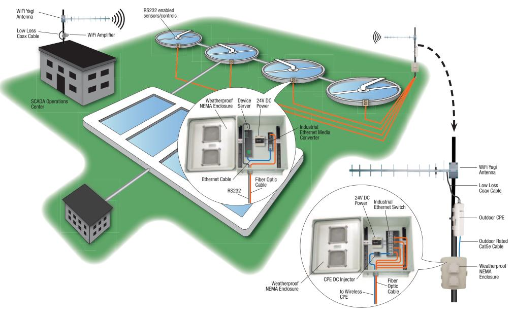
This diagram depicts a typical wastewater treatment plant network which encompasses Industrial Ethernet, RS232, and 802.11 WiFi connectivity providing an end to end wastewater treatment network solution.
