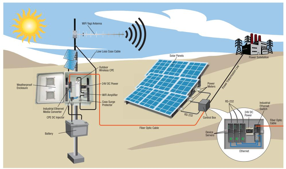
This diagram is representational only and depicts a typical solar energy network application. The diagram encompasses Ethernet, RS-232, and WiFi connectivity to provide an end to end solar energy networking solution.
