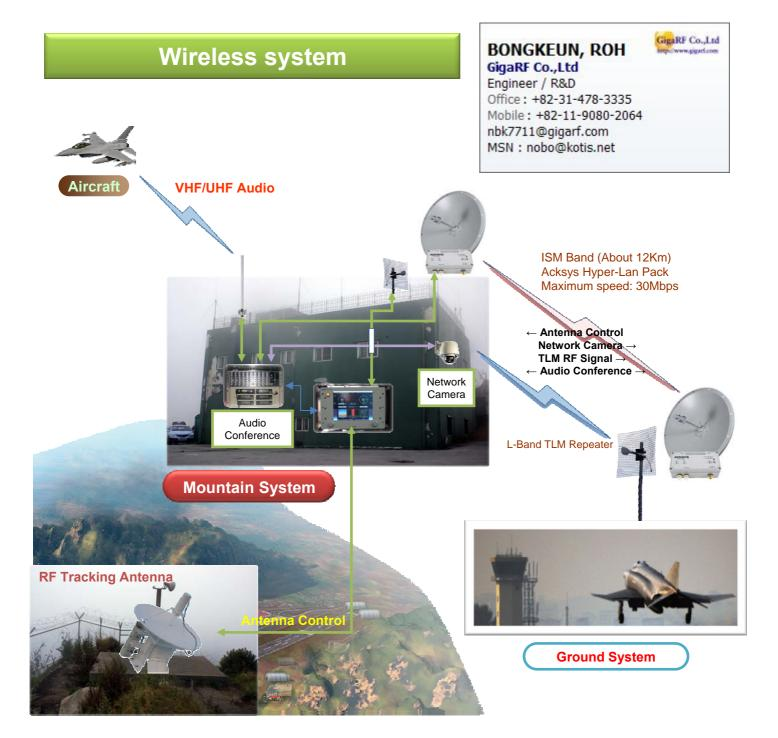
This Block diagram shows our real application using the ACKSYS HyperLan-Pack Wireless BackHaul.
