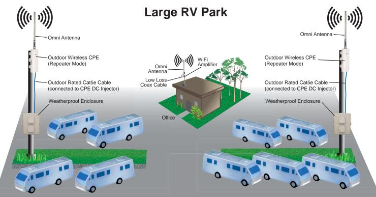
This diagram is representational only and depicts a typical RV Park WiFi application. Each wireless installation is unique and results can vary due to many different environmental factors. For outdoor wireless networks Line of Sight (LOS) must be considered. Basically that means you will need a clear unobstructed view of the antenna from the remote point in the link. Trees and leaves are obstructions to 802.11 frequencies so they will partially or entirely block the signal.
