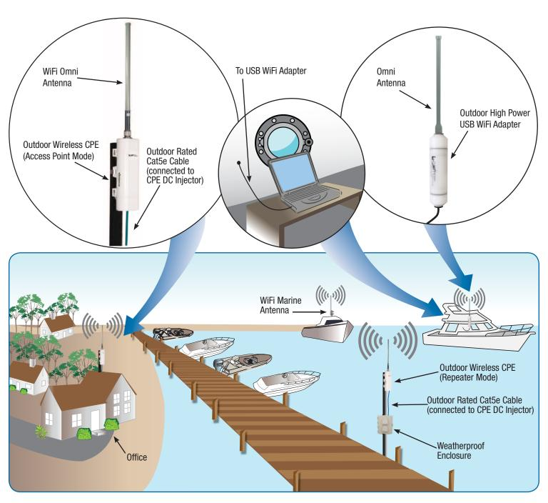
This diagram is representational only and depicts a typical Marina WiFi application. Each wireless installation is unique and results can vary due to many different environmental factors. For outdoor wireless networks Line of Sight (LOS) must be considered. Basically that means you will need a clear unobstructed view of the antenna from the remote point in the link. Trees and leaves are obstructions to 802.11 frequencies so they will partially or entirely block the signal.
