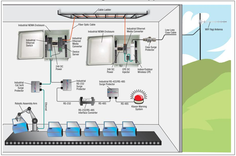
This diagram is representational only and depicts a typical manufacturing network application. The diagram encompasses Ethernet, RS-232, RS-485, and WiFi connectivity to provide an end to end manufacturing network solution.
