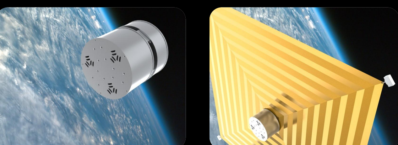
c) CHAD achieves minimum separation distance d) Web is deployed and stabilised via active control
