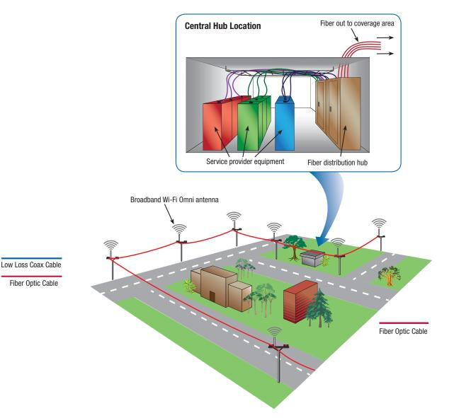
A Distributed Antenna System (DAS) involves the use of several antennas as opposed to one antenna to provide wireless coverage to the same area but with reduced total power and additional reliability. A DAS is used to provide wireless coverage to hotels, subways, airports, hospitals, businesses, and roadway tunnels etc. The wireless services typically provided by a DAS include PCS, cellular, Wi-Fi, police, fire, and emergency services.
