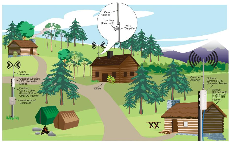
This diagram is representational only and depicts a typical campground WiFi application. Each wireless installation is unique and results can vary due to many different environmental factors. For outdoor wireless networks Line of Sight (LOS) must be considered. Basically that means you will need a clear unobstructed view of the antenna from the remote point in the link. Trees and leaves are obstructions to 802.11 frequencies so they will partially or entirely block the signal.
